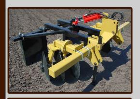
Standard Duty includes 4"x6" tool bar, Cat. II-III & stand, 11/2" square axle with trunnion mounted bearings.
